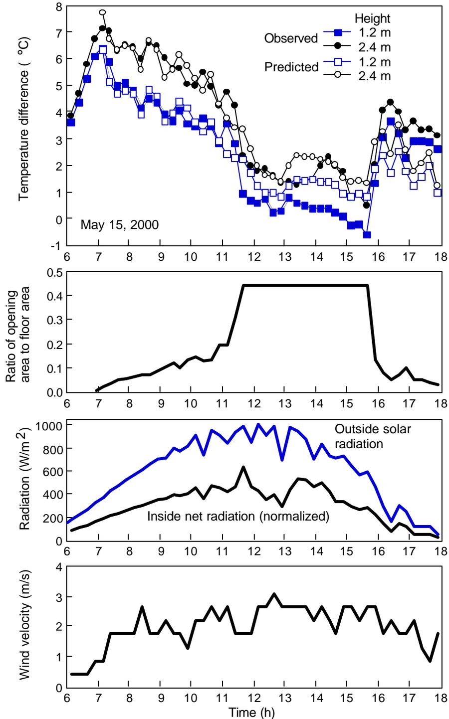
Figure 4. Comparison of the diurnal changes in predicted and observed temperature differences between inside and outside. The changes in the input parameters used for the model predictions are also illustrated.
