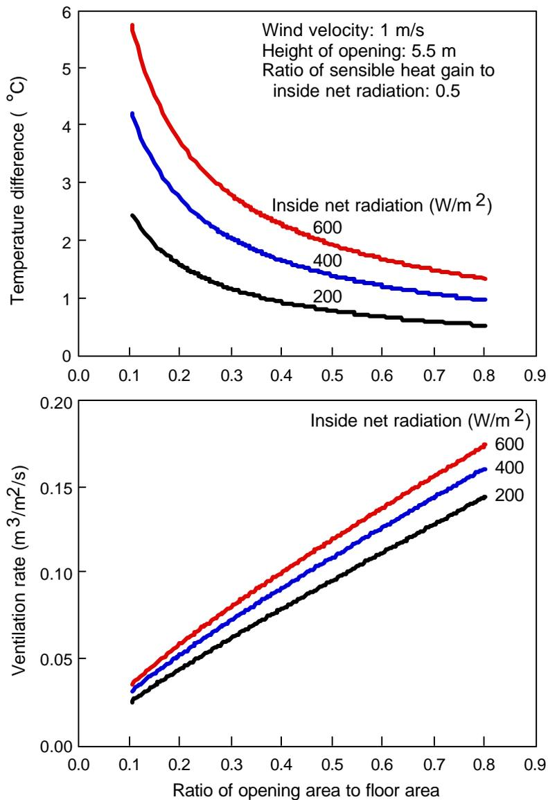
Figure 6. Predicted effects of the opening area and the inside net radiation on the temperature difference and the ventilation rate.
