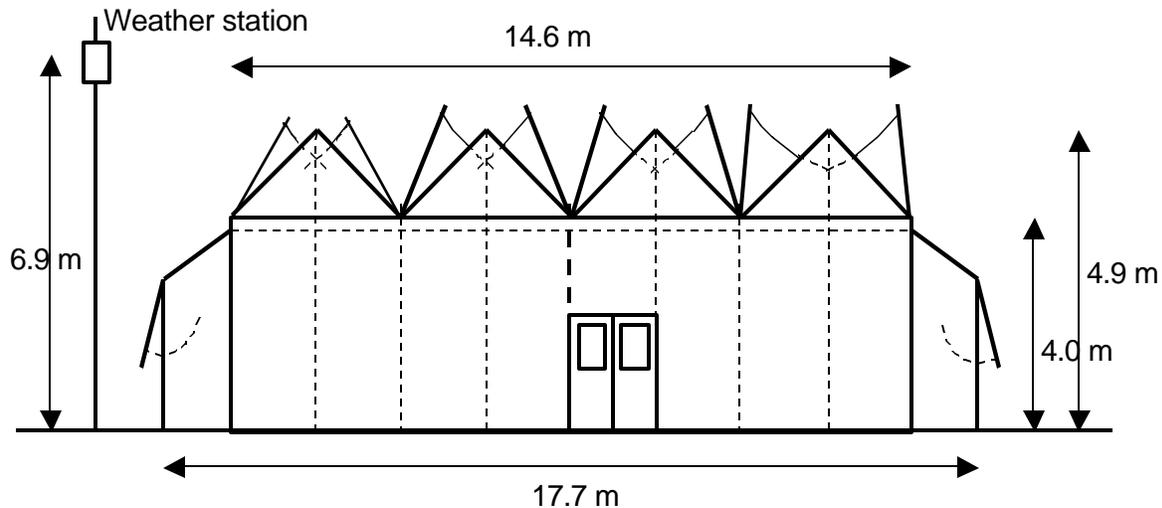
Figure 1. Side view of the greenhouse south wall (not to scale).
