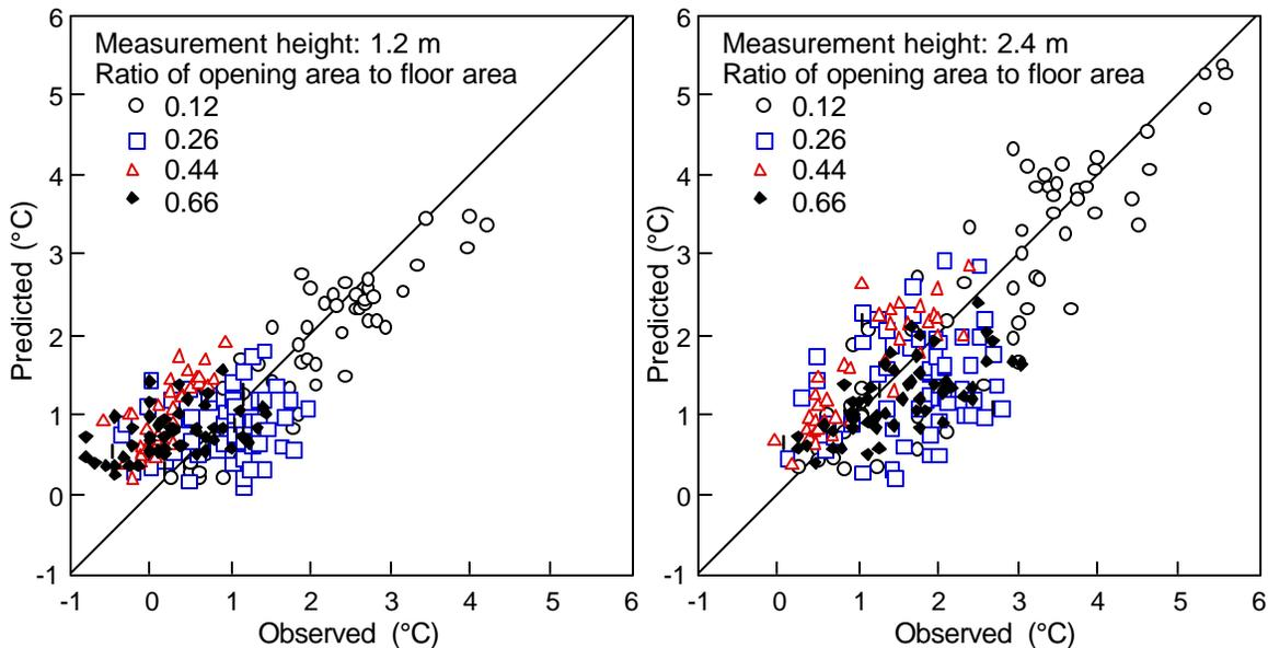
Figure 5. Comparison of observed and predicted temperature differences for four ratios of opening area to the floor area: 0.12, 0.26, 0.44 and 0.66.
