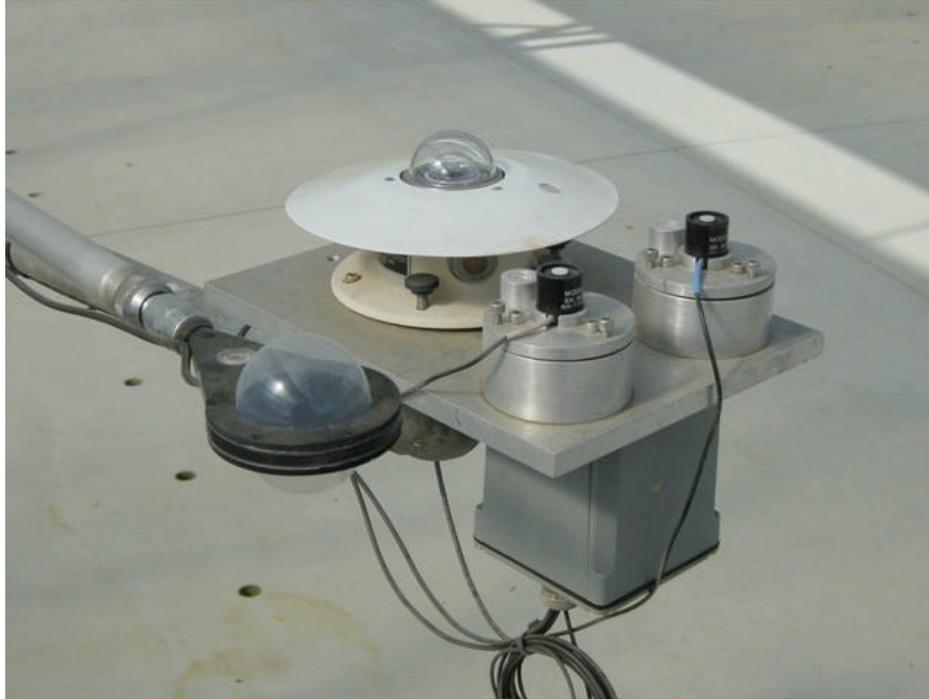
Figure 3. View of the placement of the radiation sensors inside the greenhouse.
