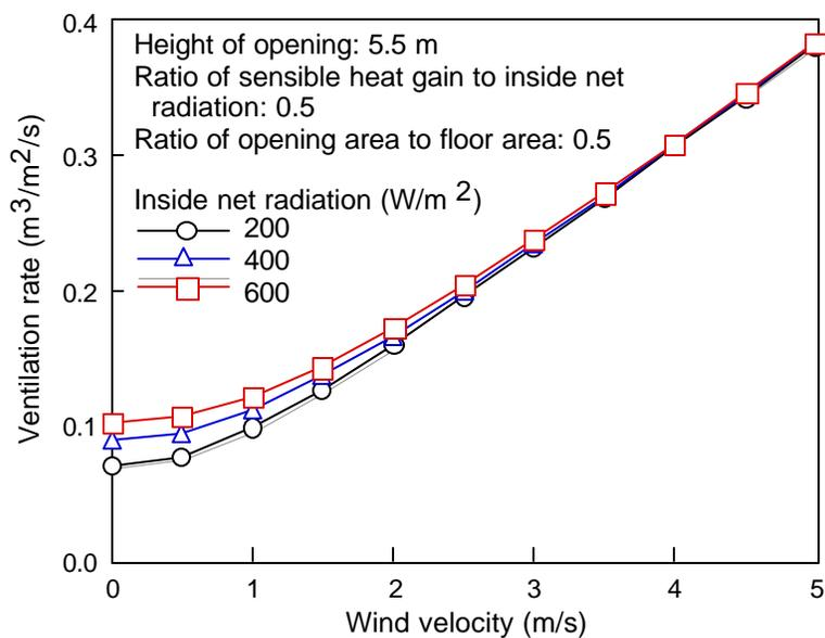
Figure 7. Predicted effect of the outside wind velocity on the ventilation rate using a constant ratio of opening area to floor area (0.5).
