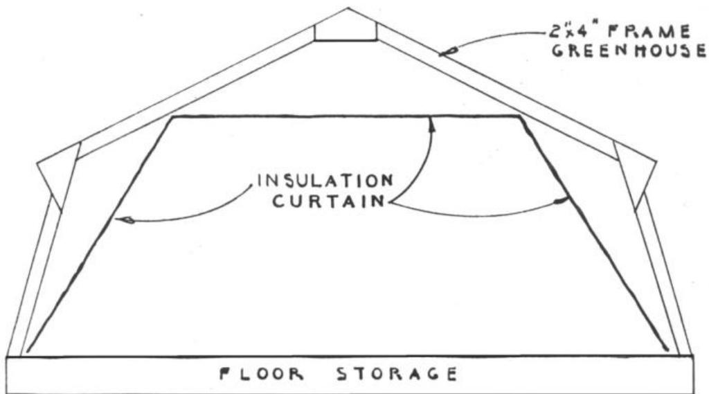
Fig. 2 Planar Insulation System for Small Prototype Greenhouse
