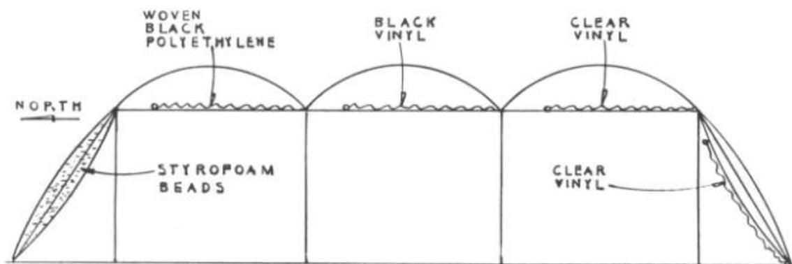
Fig. 3 Curtain Insulation System in Vegetable Production Greenhouse
