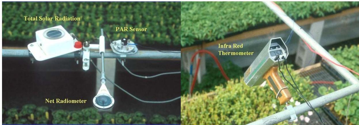
Radiation sensor array inside the greenhouse that measure: Total solar spectrum, PAR and net thermal radiation from crop canopy
