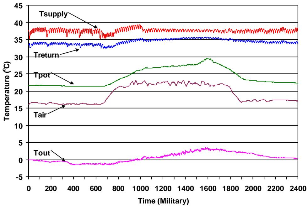
Figure 4. Third strategy, constant inlet pipe temperature of 38 °C (100 °F).
