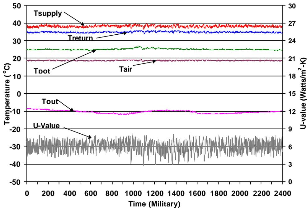
Figure 6. Data showing constant conditions during which the floor U-value was determined.
