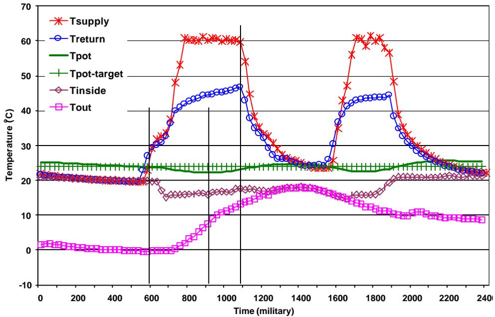
Figure 1. Control of pot temperature by floor pipe water temperature.
