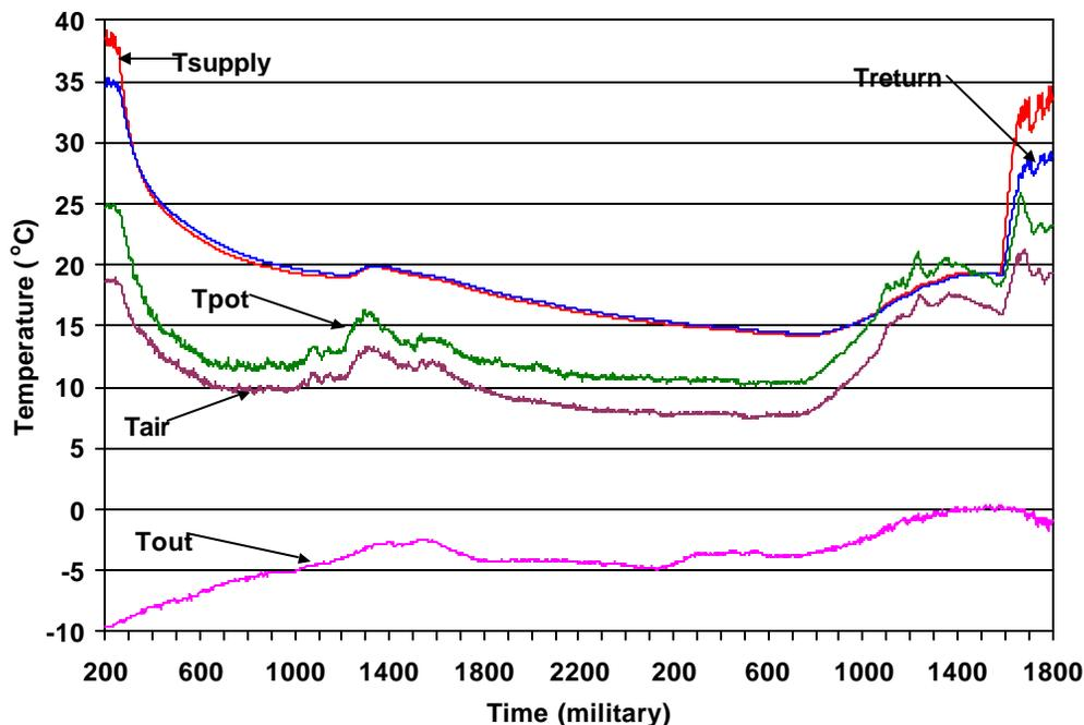
Figure 5. Data showing result of boiler failure on Feb 17, 2003.
