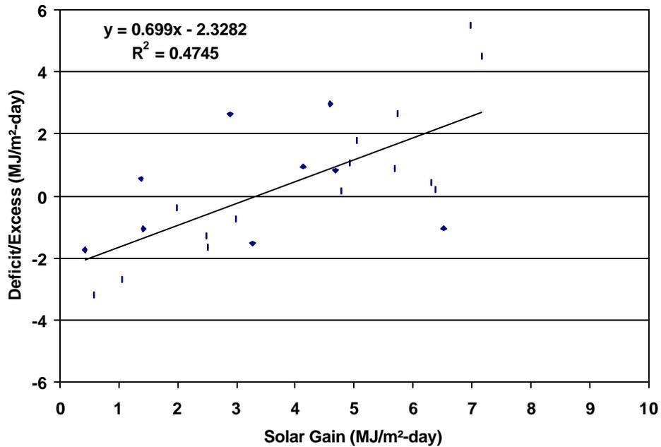
Figure 10. Daily deficit/excess of the heat provided to the greenhouse versus daily integral of inside solar radiation (third strategy).
