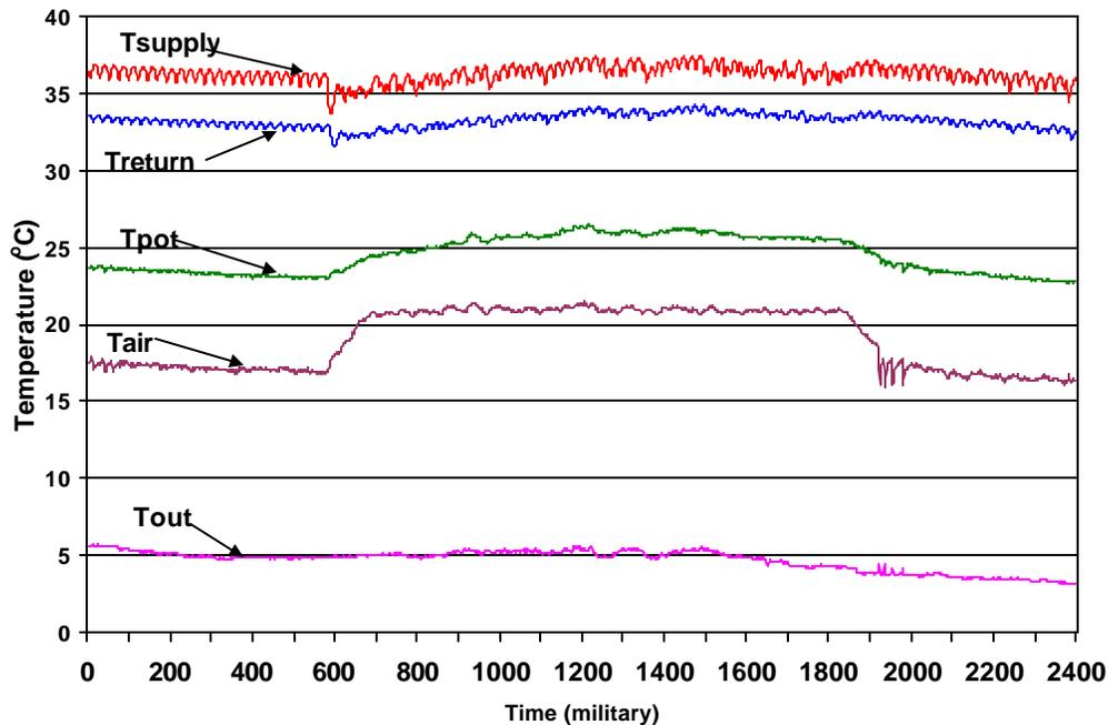
Figure 2. Effect of greenhouse air temperature on pot temperature.
