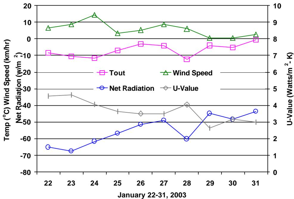
Figure 11. Effect of wind speed and radiation loss on the greenhouse U-value.
