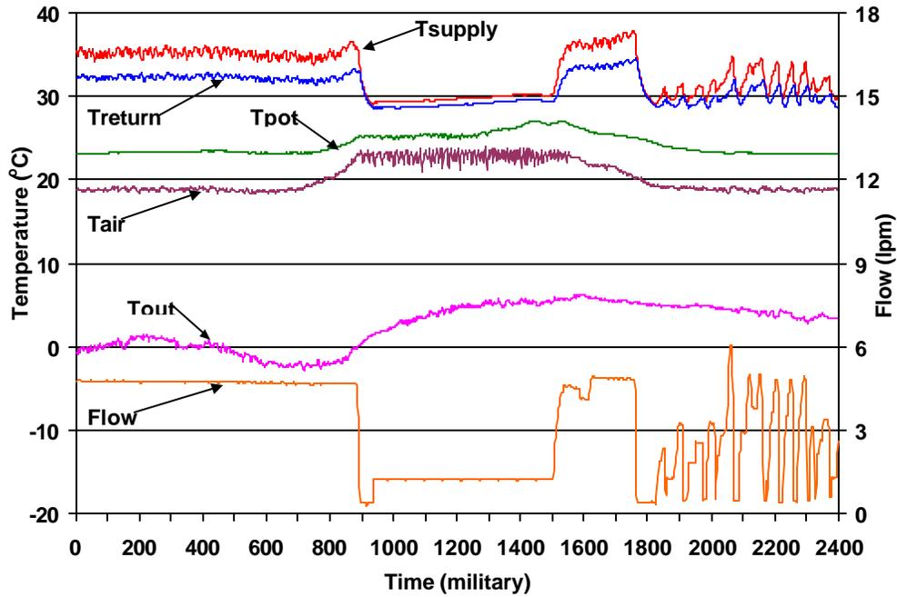
Figure 3. Second strategy, controlling air temperature by pipe water temperature.
