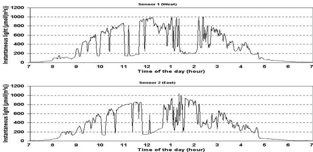
Figure 3. Instantaneous light levels measured with two light sensors in two different locations inside a greenhouse and for a 12-hour measuring period. Note that the sensors are, for the most part, not shaded at the same time so that their averaged reading gives a better approximation of the overall light environment in the greenhouse.
