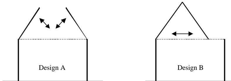
Figure 1. Two different designs of open-roof greenhouses.
