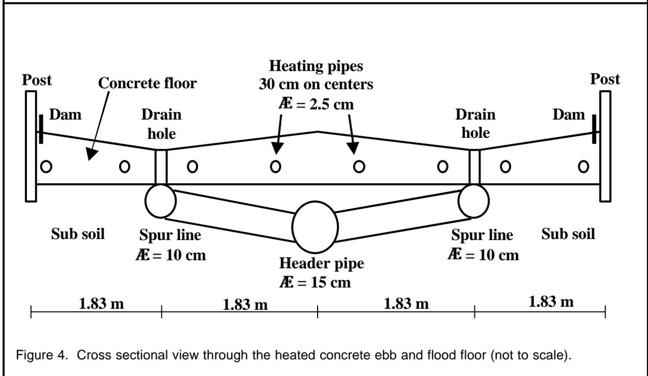
Figure 4. Cross sectional view through the heated concrete ebb and flood floor (not to scale).
