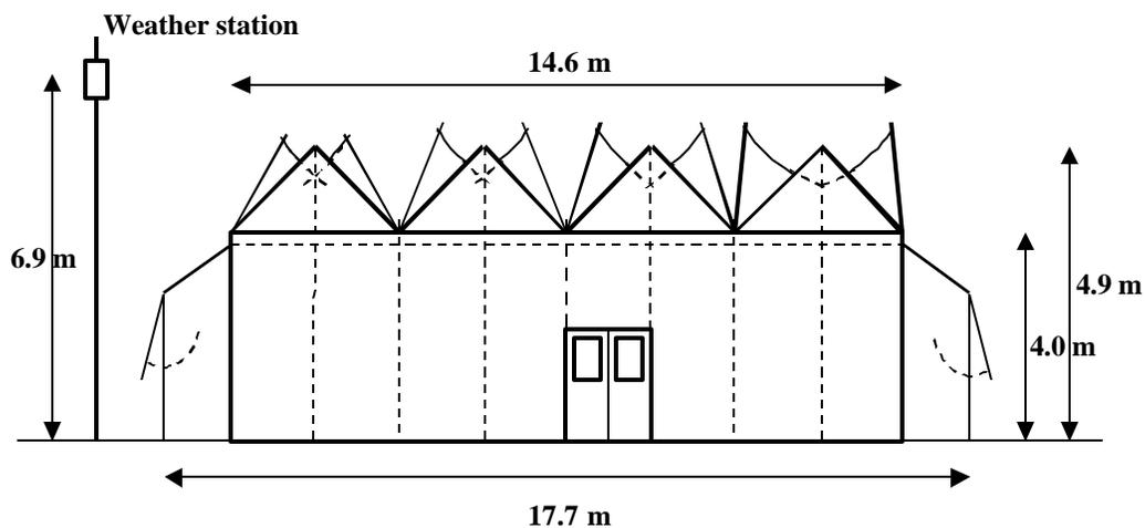
Figure 2. Side view of the greenhouse south wall (not to scale).
