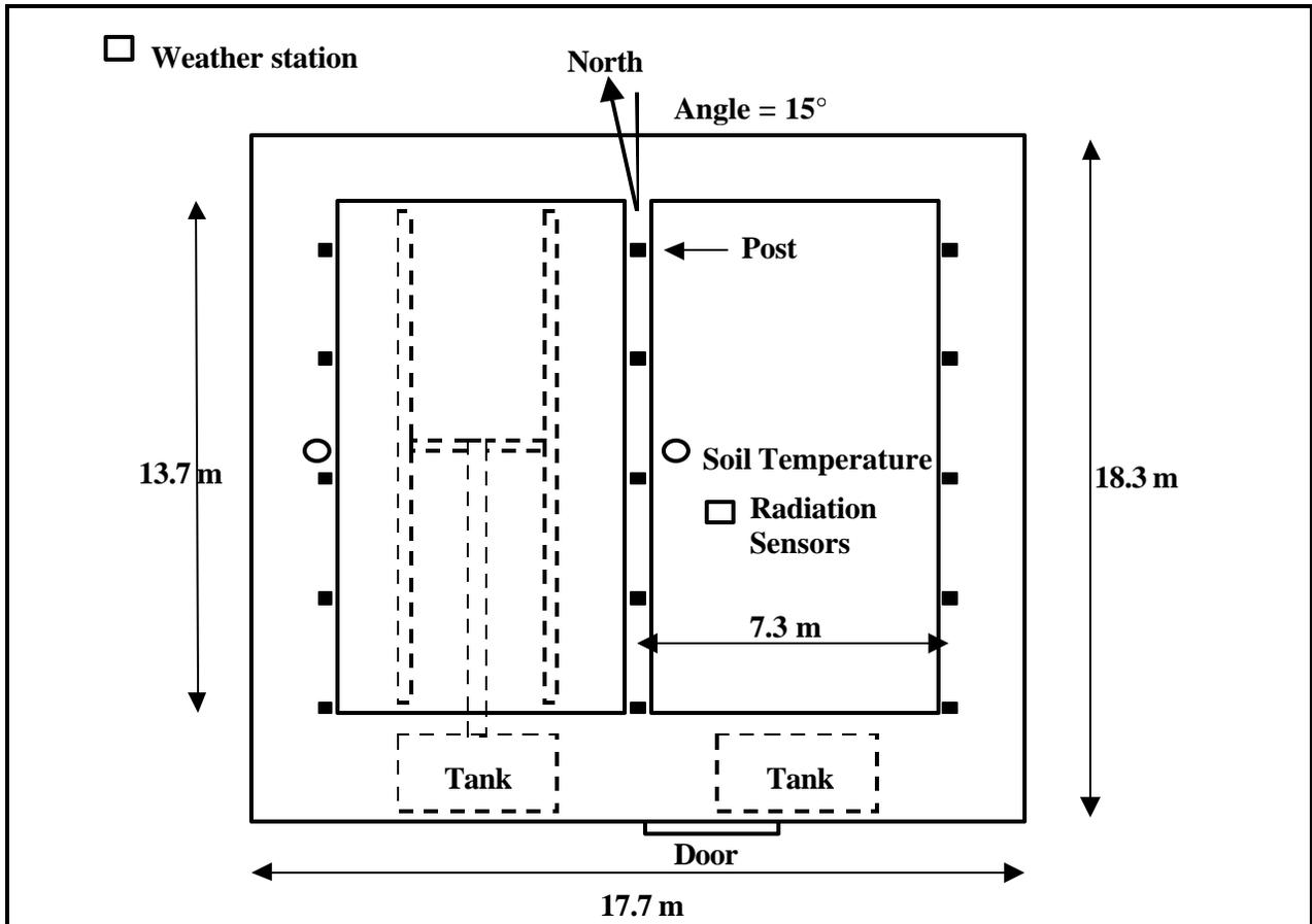
Figure 3. Greenhouse layout (not to scale).
