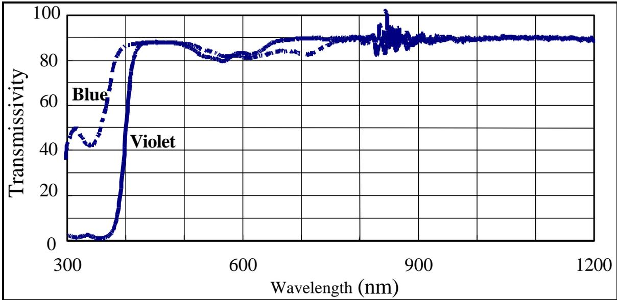
Fig. 3. Transmissivities of two different films
