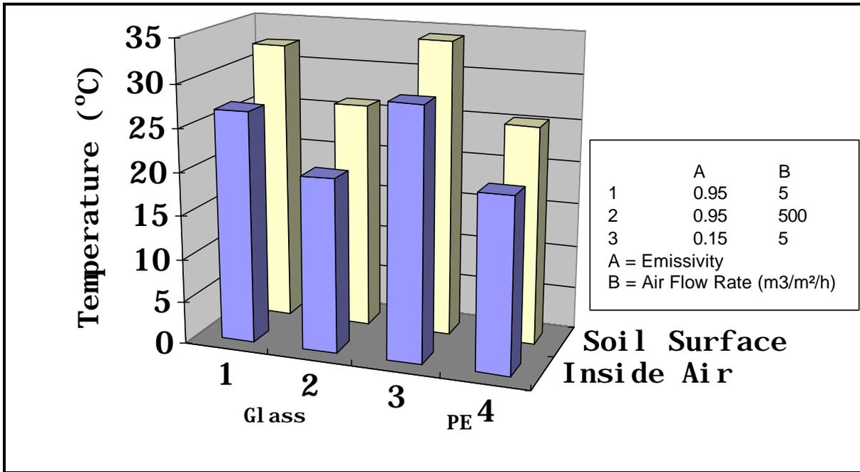
Fig. 1. The effect of emissivity of the cover and air flow rate on maximum inside air and soil surface temperatures.
