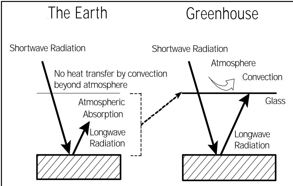
Fig. 2. Greenhouse effect in the global environment is not the same as the greenhouse effect in the greenhouse.
