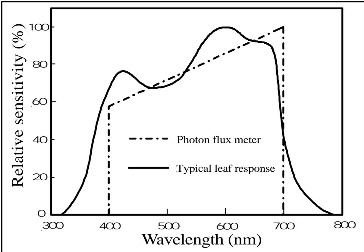
Fig. 4. Relative sensitivities of photon flux meter and average leaf response to photosynthesis.
