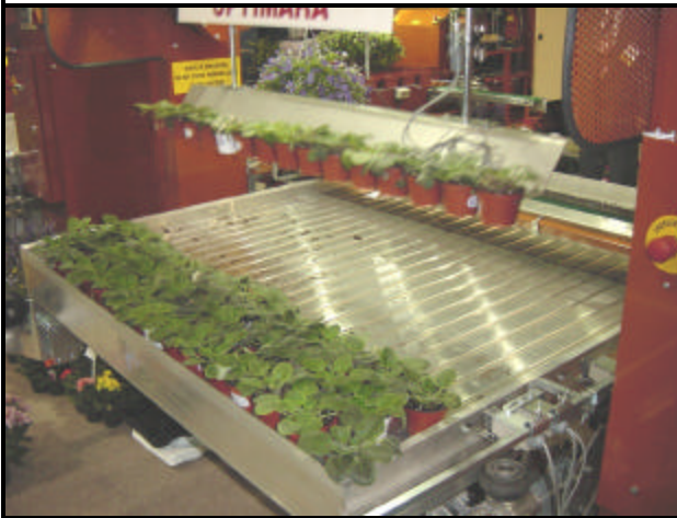
A transplanting robot moving African violets from an ebb and flood table onto a conveyor belt.
