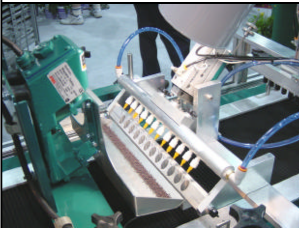
A transplanting robot moving African violets from an ebb and flood table onto a conveyor belt.
