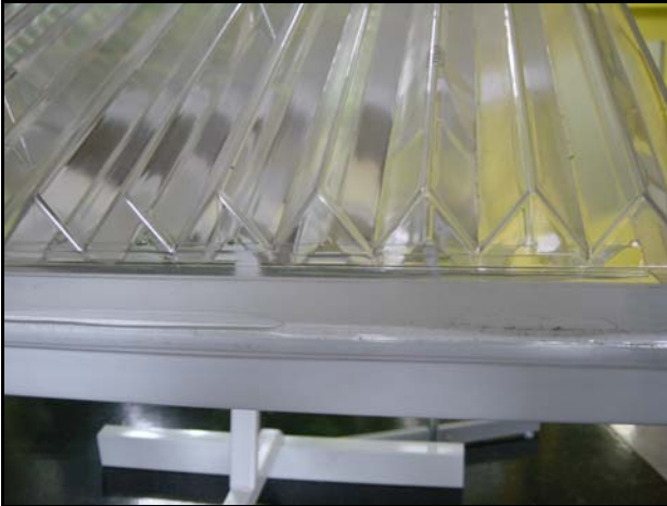
Photo 8. Twin-walled zigzag polycarbonate roofing panels. The triangular shaped ridges have base angles of 48^\circ ( 84^\circ at the top of the triangles).
