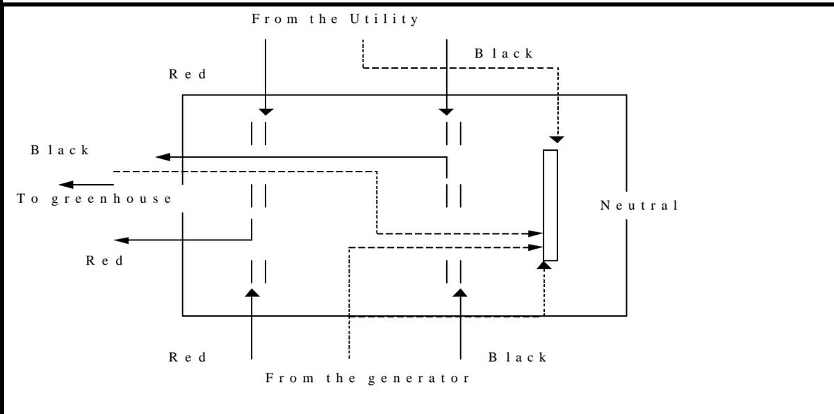
Emergency Generator System Switch Diagram of a Double pole - Double throw switch. Neutral lines are attached to a common bond. If three phase power is used, a triple pole — double throw switch is required.
