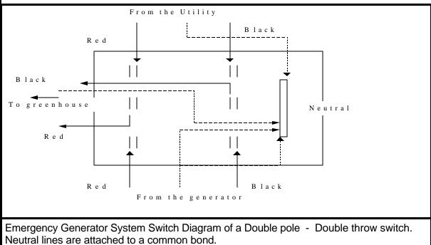
If three phase power is used, a triple pole — double throw switch is required.
