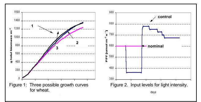
crop mass is estimated by entering current and past environmental conditions to the crop models. The control then minimizes the differences between desired (i.e., produced under nominal conditions) and the current crop total and yield biomass (which is simulated by using the crop models). A new set of environmental inputs, to be applied for the following day, is obtained through this minimization.
