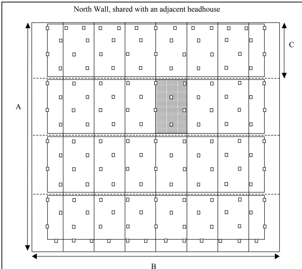
Figure 1. Design of a supplemental lighting system using 144 HPS luminaires (with 600 watt lamps) to provide a uniform light intensity of  $200 \mu\text{mol}\cdot\text{m}^{-2}\cdot\text{s}^{-1}$  over the entire growing area (mounting height = 3.2 m, A = 25.6 m, B = 29.3 m, and C = 6.4 m).
