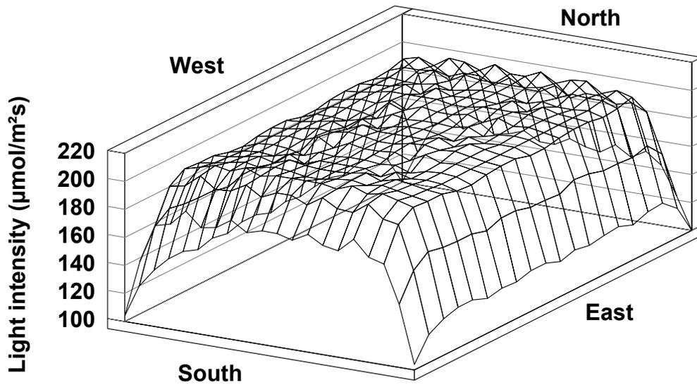
Figure 2. Light intensity for the entire lettuce growing area (25.6 by 24.1 m) as calculated with the lighting design software package Lumen Micro. The 400 light intensities were calculated in steps of 1.35 m in the E-W direction and 1.27 m in the N-S direction.
